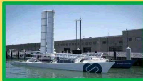
HYDROGEN POWERED BOAT ( ENERGY OBSERVER), SAME FUEL CELL IN TOYOTA MIRAI SEDAN
