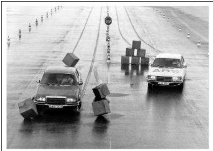
Figure 1: Left Car Uses Mechanical Brake and Right Card Uses ABS
