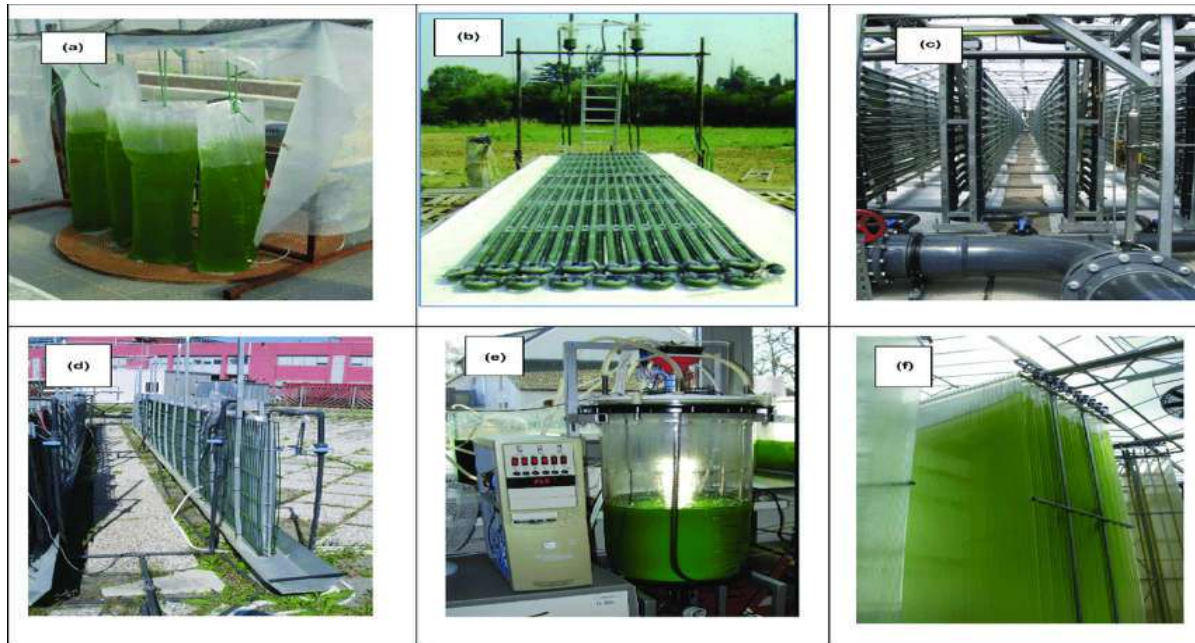
Fig. 4: Closed or semi-closed photobioreactor
